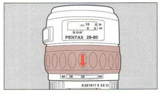
Using the manual zoom function with an FA zoom lens attached
