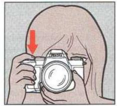
Focus [[]] on the subject. Depress the shutter release button halfway to lock focus, and then depress it fully to take a photo. (See page 35.)
