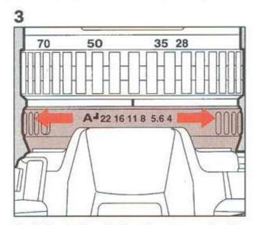
3. Adjust the desired aperture by lens aperture ring.
