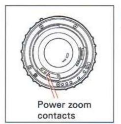
An FA zoom lens without the power supply contacts are shown in the illustration does not have the power zoom function (ie: FA28 - 70mm f / 4 AL lens).
