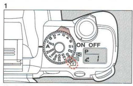
The desired metering mode, multi(6)-segment metering, spot metering or center weighted metering mode can be selected.
