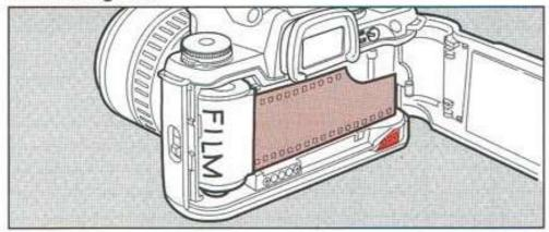
Open the back cover, insert a roll of film, align the end of the film leader with the red mark, and close the back cover. The film should advance to the first frame automatically. (See page 22.)
