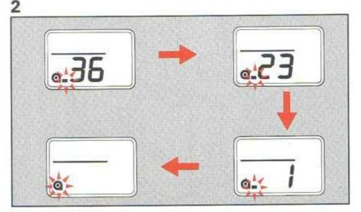
When the film is fully rewound, only [Q] blinks on the LCD panel. 3
