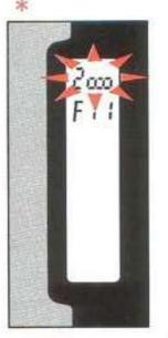
will come out 1 stop overexposed, set the lens aperture ring to [ A ] or adjust the exposure deliberately 1 stop under.
