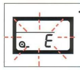
If the film is not loaded properly, [ Q\_ E ] on the LCD panel blinks, indicating that the film is not loaded properly. Open the back cover and load the film once again. 5
