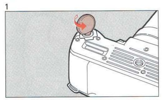
1. Open the battery chamber cover by using a coin, etc. as shown in the illustration.
