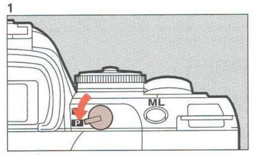
You can switch between the panorama format and standard format picture taking mode in the middle of the roll by moving the panorama lever. The panorama format picture allows horizontally positioned dynamic pictures to be taken (the panorama format is approximately 13x36mm on the film).
