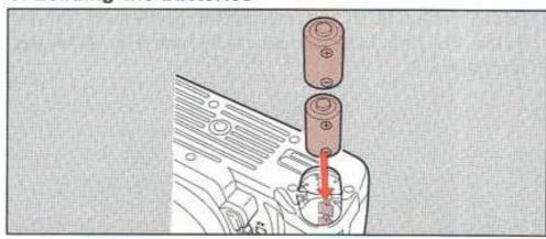
Open the battery chamber cover by using a coin. Load two batteries (CR2 type) according to the markings (+,-) in the battery chamber. (See page 13.)
