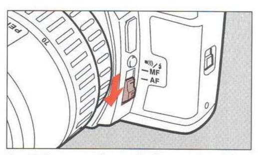
For autofocus operation, set the focus mode switch to AF .
