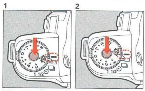
This camera automatically reads the film speed from the film's DX code. However, the film speed setting can be changed. If you use a non-DX coded film, set the film speed manually.
