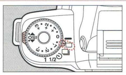
One picture is taken each time the shutter release button is depressed.
