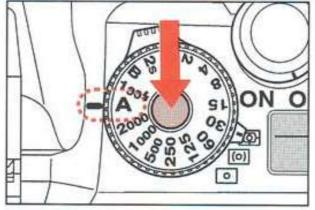
While holding down the shutter dial lock button, turn the shutter dial to [A]. (See page 26.). The exposure mode will be set in the Programmed AE Mode.
