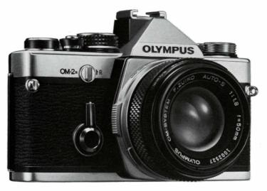
The OM-2 will not function without battery power. If you release the shutter without batteries or with batteries that are dead, the mirror locks and the field of view through the viewfinder darkens (indicating that no batteries are loaded or that the batteries are dead). To unlock the mirror load fresh batteries and move the selector lever to the CHECK-RESET position.
