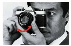
Looking through the viewfinder, rotate the focusing ring in either direction until the split images of the subject in the central spot are aligned.
